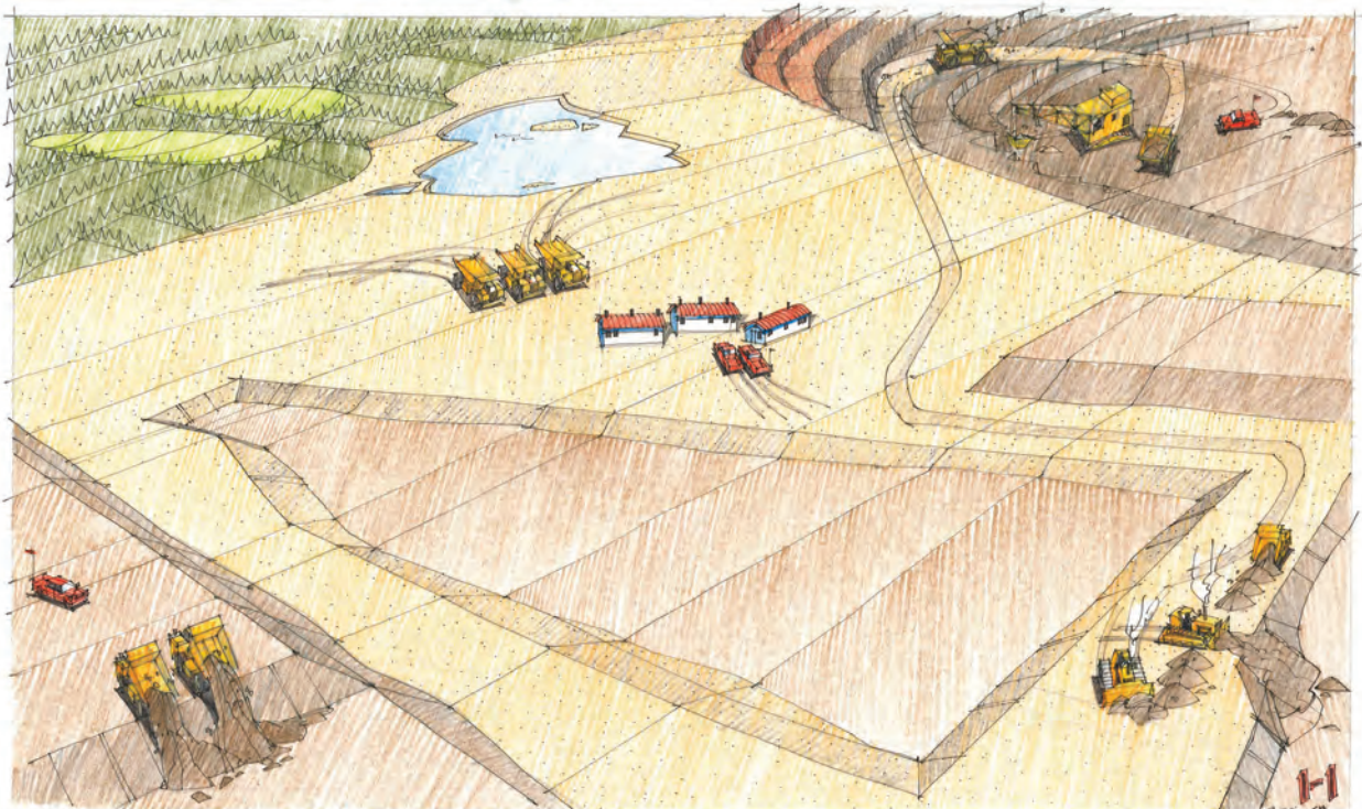
Figure 1-2. Stage 1 in the life of an oil sands mine reclaimed wetland: Initial earthworks required to rough in the wetland. The location, approximate size and shape of the wetland have been established.
